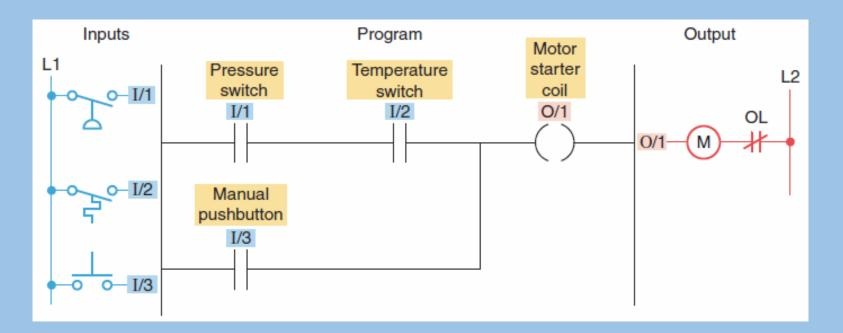
Enter the logic into the CPU processor program
